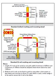
to be used to secure the U-rail in the sleeve. 3. Where a U-rail is mounted at right angles to a path a 'target board' shall be fitted. If the U-rail is mounted longtitudinally along the path a target board is not used. See inset for 'target board' detail.
